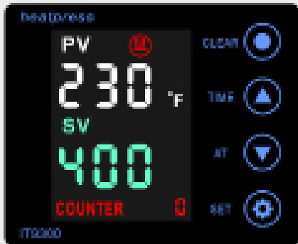
User can wake up heat press and start heating by touching any key
