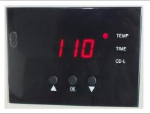
Press m button, the temp light light is ON. Press Up " $\triangle$ " or Down " $\nabla$ " button to set temperature according to different transfer material. (Normally  $180^{\circ}\text{C}\sim200^{\circ}\text{C}$ )
