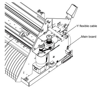
(7) Remove the Y-flexible cable attached with double-sided adhesive tape to the Y-rail.
