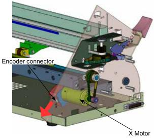
Mount the X motor that the encoder connector of X motor to be faced to the front.
