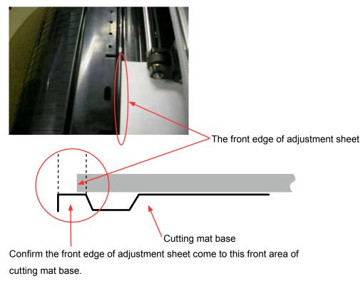
(15) Press the ENTER key after confirmed the position of front edge of adjustment sheet.
