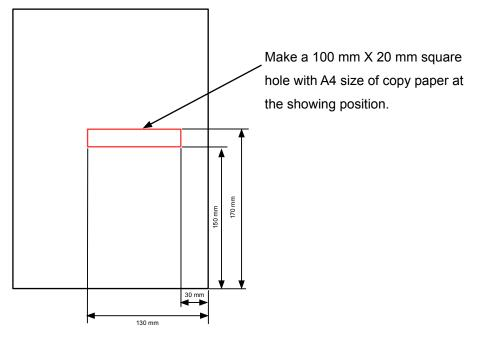
The adjustment target sheet does not need to make if the recorded adjustment values are input.
