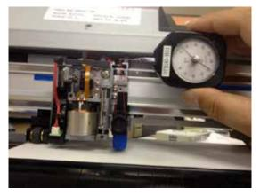
The measured pen force should be within the specification range (10±2 g).
