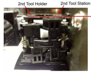
The height of 2nd tool holder should be same level to the 2nd tool station.
