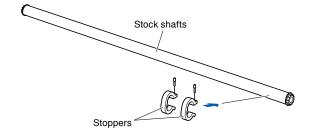
(2) Put the stock shaft into the media stocker as shown in the picture below.
