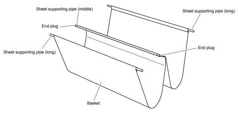
(7) Using the middle sheet supporting pipe, attach the basket assembly from step 6 to the media stocker, then attach the joints from the assembly from step 5 to the long sheet supporting pipe from step 6. The middle of the basket should pass over the back end of the center bar.
