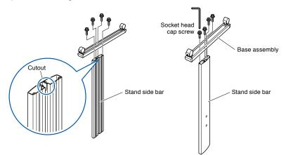
(2) Loosely fasten the center bar to the left and right stand sides with four socket head cap screws (two on each side), using the Allen wrench. Mount the center bar so that each one of stand feet of short side to be front side.
