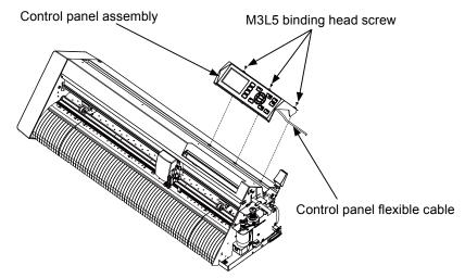
(4) Disconnect the LCD flexible cable from the control panel key board.
