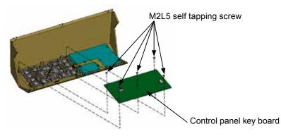
(6) Detach the control panel key board.
