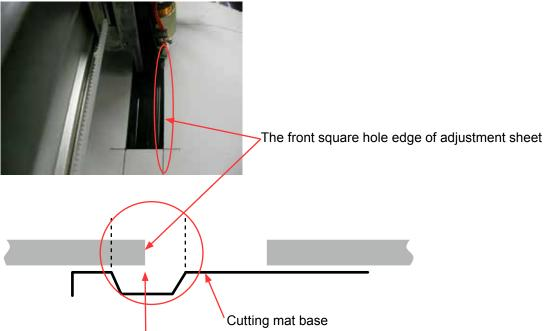
Confirm the front square hole edge of adjustment sheet come to this
