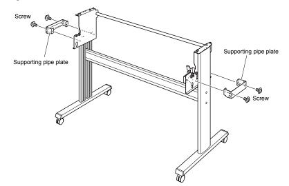
(5) Insert the 4 short sheet supporting pipes into the supporting pipe plate from the end without an end plug. In the front side of the main assembly insert the pipe into the upper side, and insert it into lower side in the rear side. The short sheet supporting pipe ends should now extend out from the front end of the main assembly.
