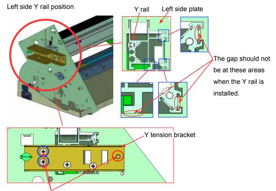
The left side of Y rail is fixing by these three screws and the Y tension bracket.
