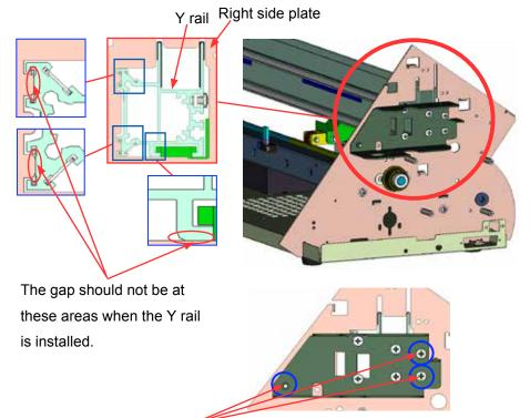
The right side of Y rail is fixing by these three screws and the Y motor bracket.
