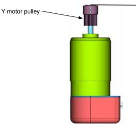
Install the Y motor pulley at the end of the Y motor shaft. So the surface of end of motor shaft and surface of pulley should be flat.
