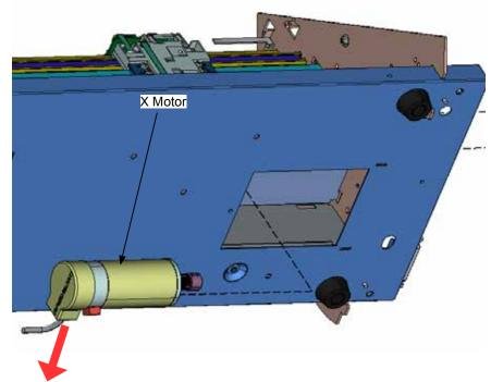
Mount the X motor that the encoder connector of X motor to be faced to the rear.
