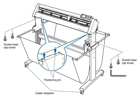
(9) Tighten the socket head cap screws loosely fastened in Step 2.
