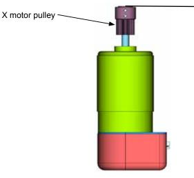
Install the X motor pulley at the end of the X motor shaft. So the surface of end of motor shaft and surface of pulley should be flat.
