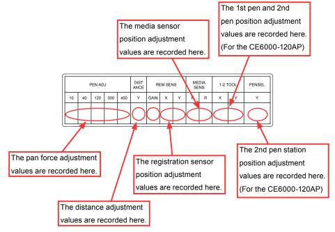
You can input the same values when you have replaced the main board without making any adjustments except the Registration Mark Sensor Sensitivity adjustment.
