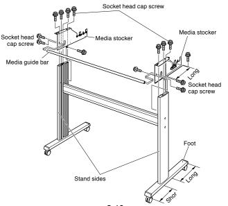
(4) Mount the plotter on the stand by inserting the positioning pins on the stand into the positioning holes on the underside of the plotter. Fasten with four socket head cap screws (two on each side), using the Allen wrench.
