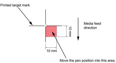
Note: Position the pen-tip to the area above. Do not position the RMS sensor to the area above.
