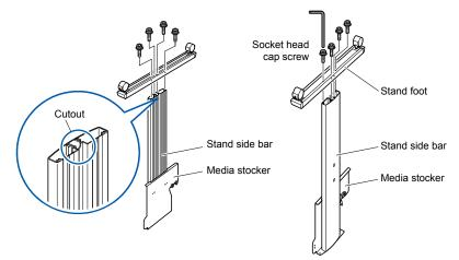
(2) Loosely fasten the center bar to the left and right stand sides with four socket head cap screws (two on each side), using the Allen wrench. Mount the center bar so that each one of stand feet of short side to be front side.
