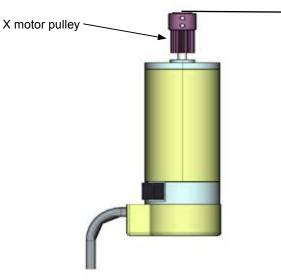
Install the X motor pulley at the end of the X motor shaft. So the surface of end of motor shaft and surface of pulley should be flat.
