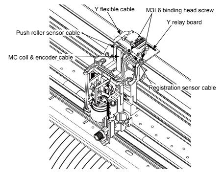
(4) Remove the two M3L6 binding head screws attaching the Y-relay board.
