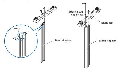
(2) Attach the center bar to each of the left and right stand sides temporarily with two socket head cap screws, using the Allen wrench. Mount the center bar so that each one of stand feet of short side to be front side.
