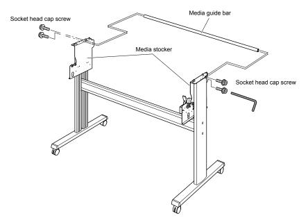
(4) Fasten supporting pipe plate to the left and the right of the stand side bar with four screws (two on each side), using the Allen wrench.
