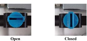
Figure 5-63. Operation of the Ink Leak Measurement Jig
