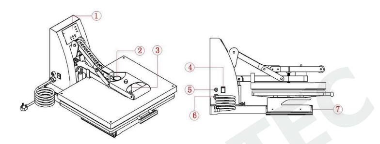
1 GY-04 Digital Controller 2 Pressure Adjust Knob ⑤ Fuse
